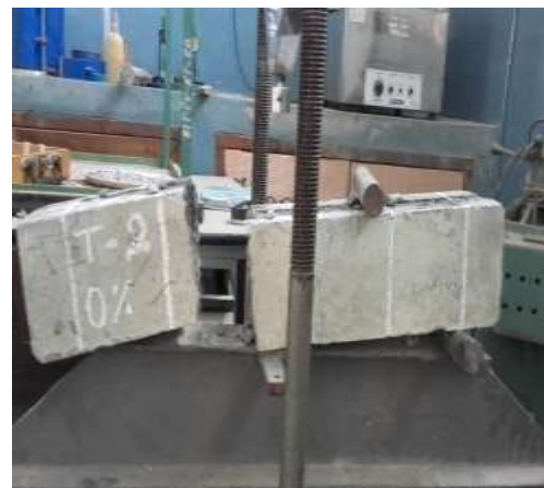
Fig 7. Prism after flexural failure
