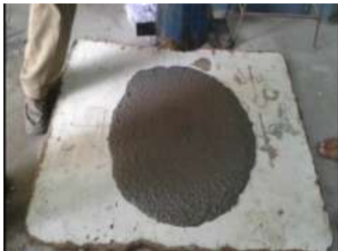
Fig.1(a). Flow before adding glass fibre
