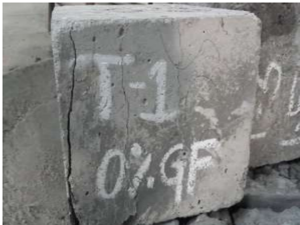
Fig 6. Cubes after compression test
