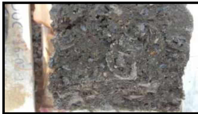
Fig 8. CS of prism failed under flexure test
